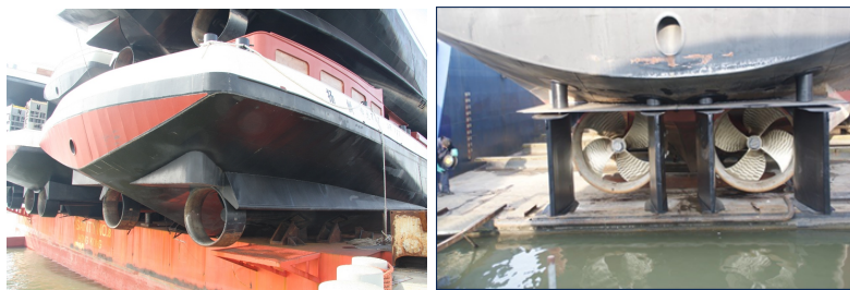
Figure 2.3: Two sterns of inland ships during repairs or maintenance (Photos by René Rapati, Groenendijk & Soetermeer)
