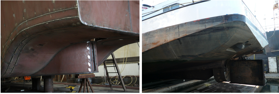
Figure 1.3: Left: Example of a pram-shaped stern, including a skeg. Right: Stern of an inland ship, including a tunnel, rudders, a propeller duct and anchor vaults. (Photos by René Rapati, Groenendijk & Soetermeer)
