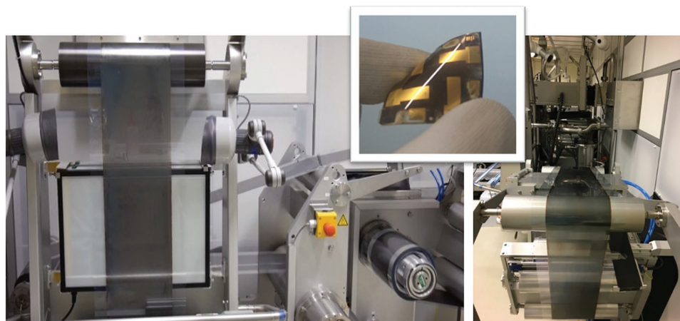
Figure 3. Photograph images of the roll-to-roll coated perovskite layer ( \text{Cs}_{0.15}\text{FA}_{0.85}\text{PbI}_{2.85}\text{Br}_{0.15} ) and an example of the manufactured flexible devices.
