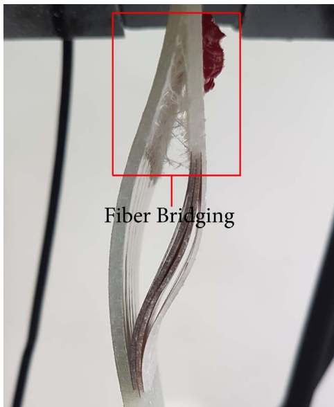
Fig. 16. The fiber bridging phenomenon in specimen S_{M-K} .
