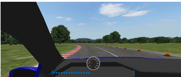
Figure 2: Outside visuals shown during the experiment, showing the white reference line drawn on the road center and the rating bar at the bottom in blue.
