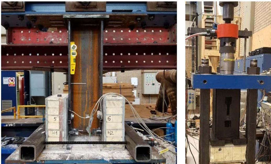
Figure 1. Push-out (left) and pull-out (right) tests
