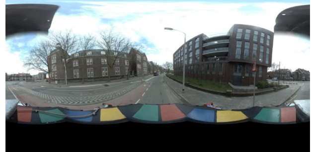
Figure 2. A panoramic image on a sphere. The lines represent latitude and longitude.
