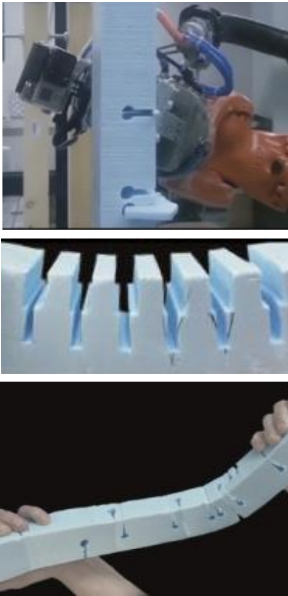
Figure 5. Materialization experiments and robotic production process involve robotic milling (top), preliminary research on the geometry of the milled section (middle) and robotically fabricated component (bottom)
