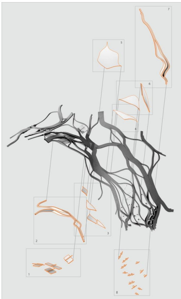
Figure 6. Fragment showing bended beams system accommodating mechatronic devices: (1) heating devices, (2) variable-depth structural elements, (3) small windows for natural illumination, (4) water storage compartment, (5) large window for illumination and views, (6) cooled-air chamber and wetted pads, (7) variable-depth structural elements, and (8) cooling devices.
