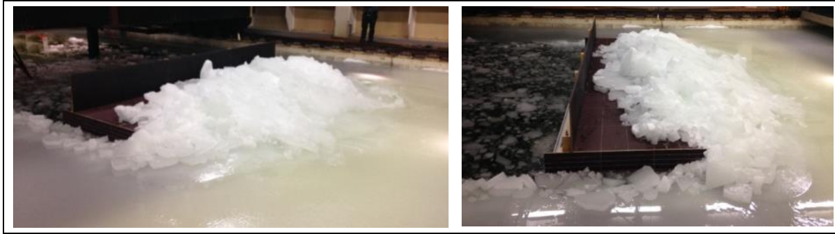
392 Figure 3-2. Images showing the final state of a model test. The structure and ice pile-up are at the 393 centre, the intact ice sheet is to the right and the open water channel to the left with loose ice pieces 394 left behind in the wake as the structure moved from left to right.
