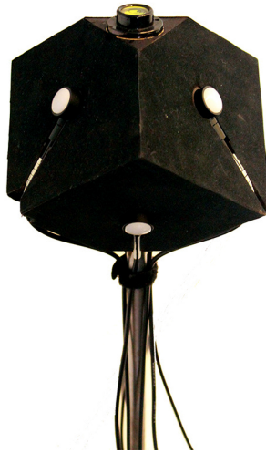
Figure 6.1: Our cubic illumination meter, built with commercially available components on the basis of a laser-cut cube basis (see Appendix C for additional materials to build this basis). Note: our cubic meter has 6 large faces and 2 small faces. The small face on the top was cut to place a spirit level and the small face on the bottom was cut to fix the cubic meter on a metal stick.
