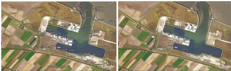
Fig. 6.52. PS targets before (left) and after (right) selection on height above ground level (5 meters). The selected PS targets correspond with buildings; the PS at lower heights are deselected.
