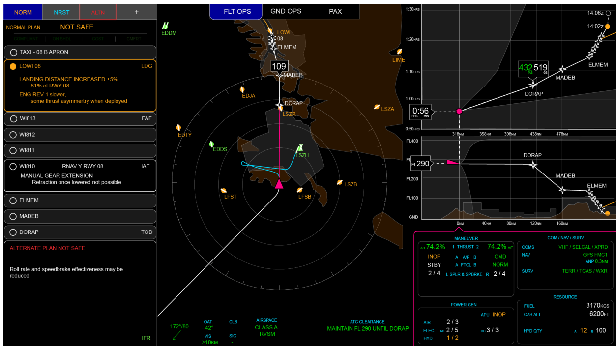
Figure 2. Flight plan evaluation concept in the non-normal condition of a hydraulic failure.
