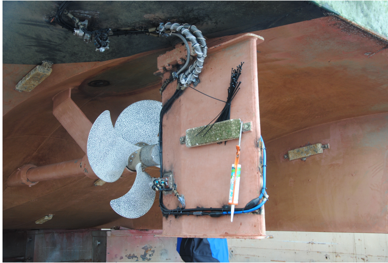
Figure 7: Lights on rudder and hull and cables.
