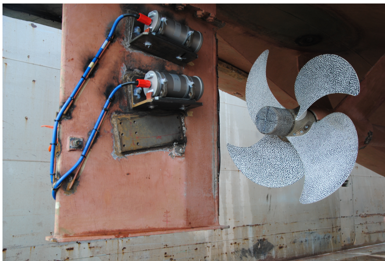
Figure 6: Starboard rudder side with cameras.
