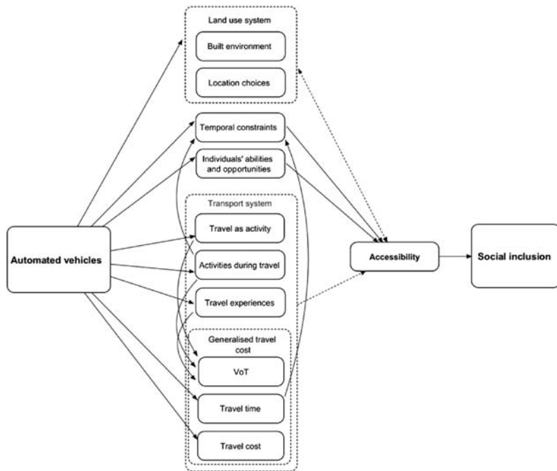
FIGURE 4.1 The conceptual model of the long-term implications of automated vehicles for social inclusion. Source: Adapted from Milakis, D., 2019. The societal dimension of the emerging mobility technologies transition: towards a research agenda. The Case of Automated Vehicles (Working paper).
