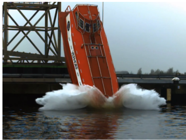
Figure 1: Drop test with free-fall lifeboat (from: www.verhoef.eu )
