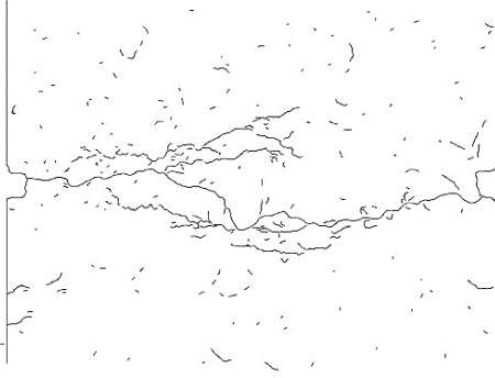
Figure 5.39 Fracture pattern for representative MSHB test on BFS cement concrete Normal (07H01).
