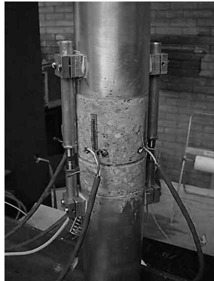
Figure 3.14 Detail of the specimen glued into the set-up.
