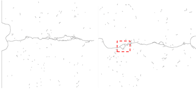
Figure 4.21 Static fracture: crack branching (test 03D2).
