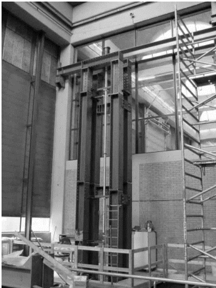
Figure 3.13 The Split Hopkinson Bar set-up at the Delft University of Technology.
