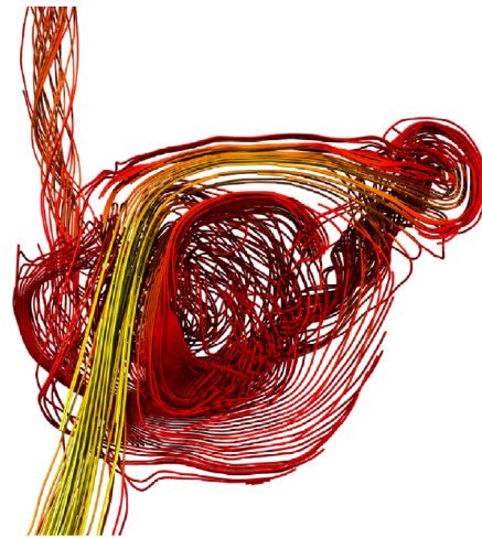
Figure 6: Streamlines of the measured flow after our method was applied. All visualization parameters (number of lines, seeding position, cutting plane and camera parameters) are equal to those in Figure 5. Note that the flow features are preserved while more streamlines are visible due to the lack of divergence and flow not leaving the segmentation.
