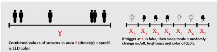
Fig. 4. Design scheme for a dynamically responsive lighting system based on automated inputs was linked real-time to user activities such as seating, walking, running.
