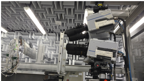
FIG. 3. Tomo-TR PIV setup.
