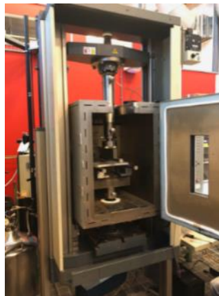
Fig. 11 3-Point bending test setup for elevated temperatures.
