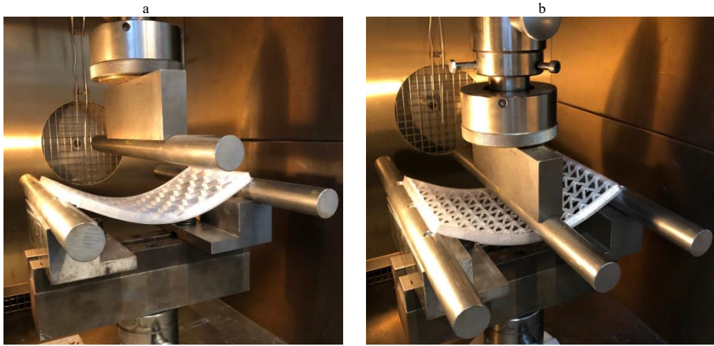
Fig. 12a) Recycled PET core with honeycomb pattern deflection without a force at 80 °C, b) Recycled PET core with truss pattern deflection at 80 °C.
