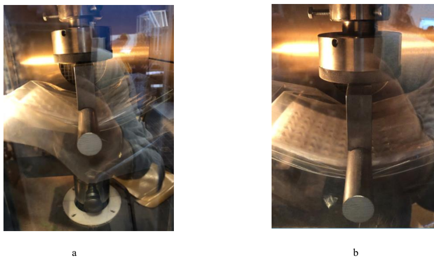
Fig. 13a) Composite panel (honeycomb core) with a deflection of 50mm at 80 °C, b) Composite panel (truss core) with a deflection of 50mm at 80 °C.
