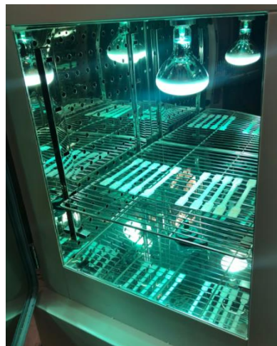
Fig. 3 Accelerated UV source with 3D printed specimens.
