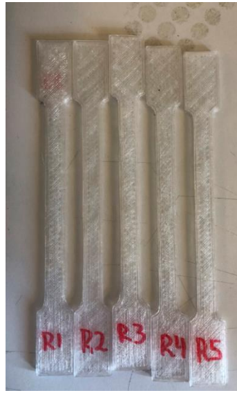
Fig. 2a) dimensions dumbbell specimens based on NEN-ISO 527-1 Standard, b) 3D printed PET specimens, c) 3D printed Recycled PET specimens.
