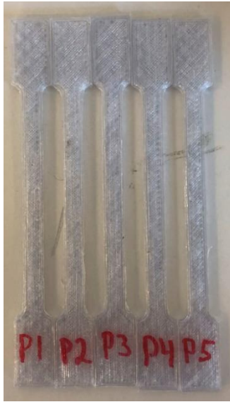
Fig. 2a) dimensions dumbbell specimens based on NEN-ISO 527-1 Standard, b) 3D printed PET specimens, c) 3D printed Recycled PET specimens.
