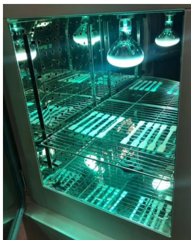
Fig. 3 Accelerated UV source with 3D printed specimens.
