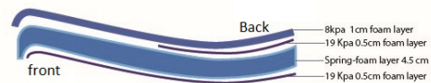
Fig. 5. Side-view of the prototype seat-pan showing the layer composition of different foams.
