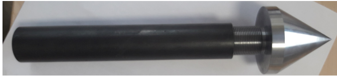
Figure 5.3: Newly developed drive point for inserting fiber-optic cables with cone penetration test equipment. Picture taken by Rolf Rekers, Wiertsema.
