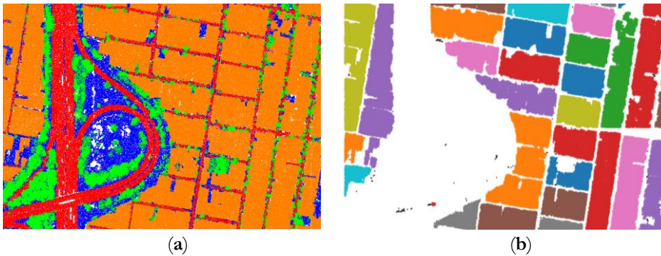
Figure 2.4 Point cloud classification and segmentation results on a small subset of Surabaya city, Indonesia. (a) Classification results in points labelled according to their classes (blue represents bare land, green represents trees, orange represents buildings, and red represents road); (b) segmentation results in different building blocks, all consisting of points having the class labels buildings (different colors indicate different building blocks).
