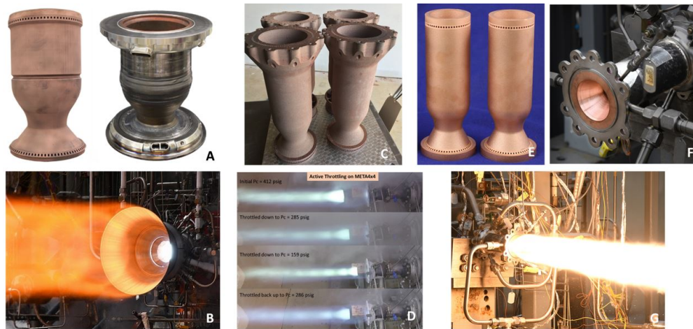
Figure 3: Various AM copper alloy chambers demonstrated by NASA and commercial partners: a) Bimetallic 156 kN using L-PBF GRCop-84 and Inconel DED, b) LOX/LH 2 Hot-fire testing of 156 kN bimetallic chamber, c) Large-scale GRCop-42 31 kN chamber, d) LOX/LCH 4 hot-fire testing of 31 kN, e and f) L-PBF C-18150 and bimetallic 10.7 kN chamber, and g) Hot-fire testing of 10.7 kN bimetallic chamber (credits NASA).
