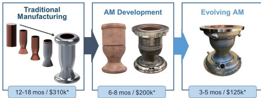
Figure 1: Comparison of traditional manufacturing to additive manufacturing evolution (cost in US$, 2020 equivalent, credits NASA)
