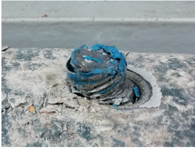
(a) Coupler with part of fractured bolt.
