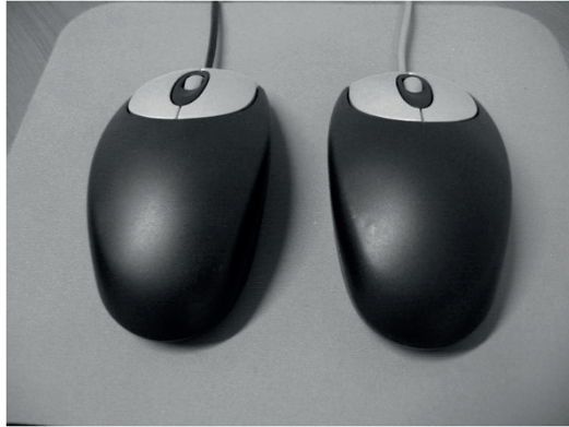
Figure 1 On the left the Hoverstop Mouse (continuous signal) and on the right the mouse with the on-off-on signal, both are identical on the outside. The mouse on the right was also used for the no-feedback condition, but then the vibro-motor was switched off
