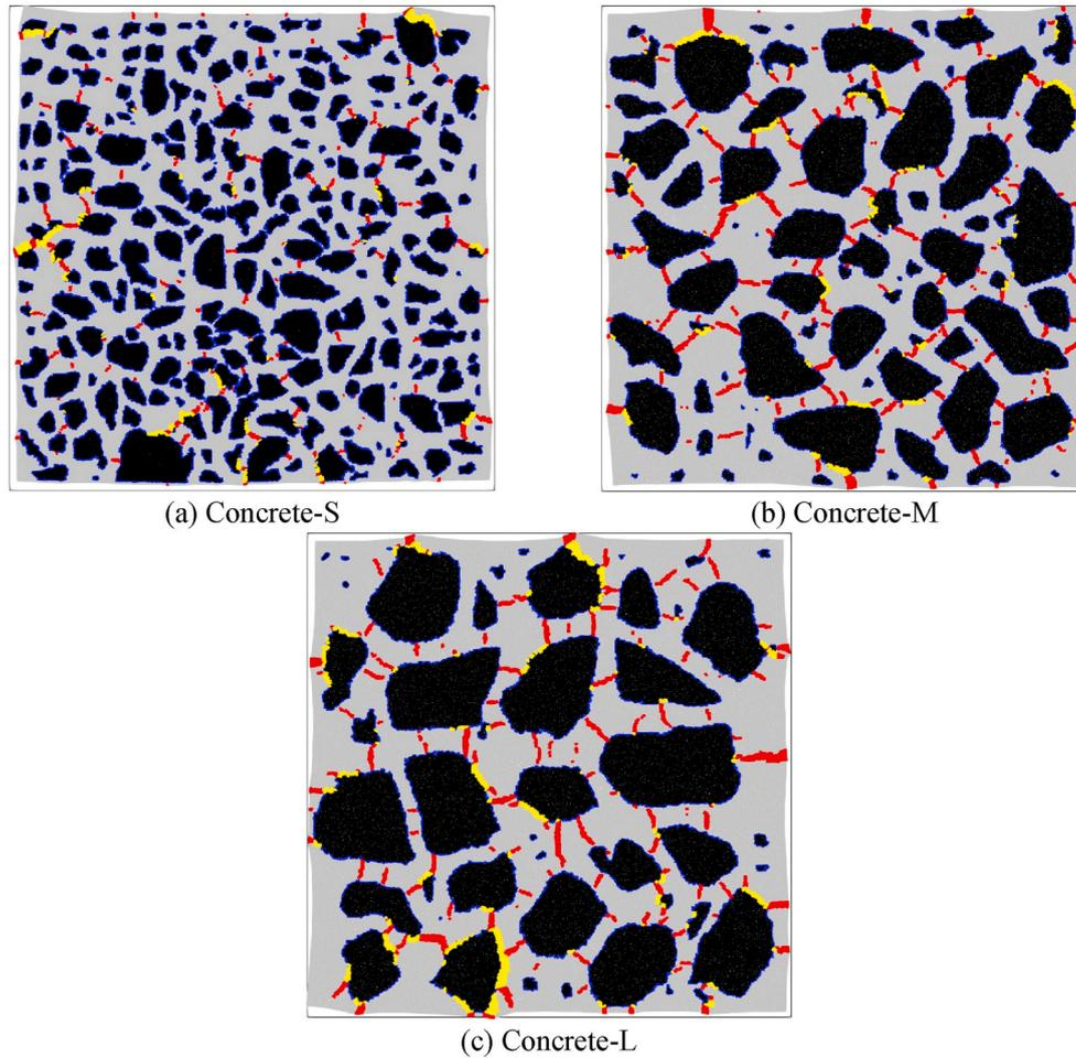
**Fig. 11.** Patterns of  $>5 \mu\text{m}$  microcracks in concrete slices under drying for 60 days (obtained using lattice fracture model): grey is mortar, blue is interface, black is concrete, red is microcrack in mortar, yellow is microcrack in interface. Deformations and microcracks are magnified 50 times. (For interpretation of the references to colour in this figure legend, the reader is referred to the Web version of this article.)
