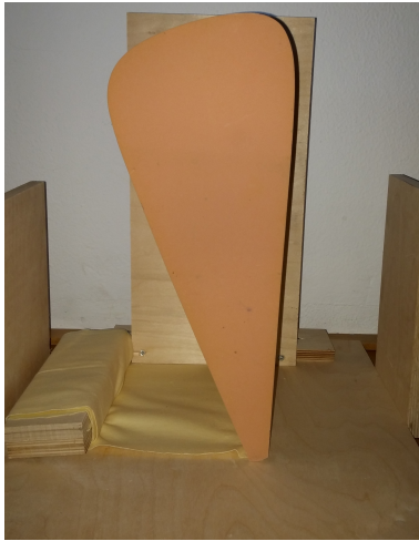
Fig. 8: One sided mould out of high-density foam material.
