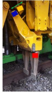
a. Multi-sensor equipped on a tamping unit in a field test (reproduced from [47])
