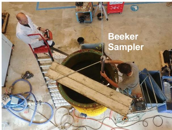
Figure B6: Deployment of the Beaker Sampler.
