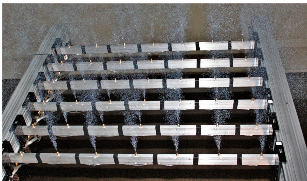
Fig. 15 NLR’s seeding rake of 42 bubble generators
