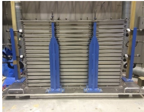
Fig. 2 Laminar soil box during sample preparation
