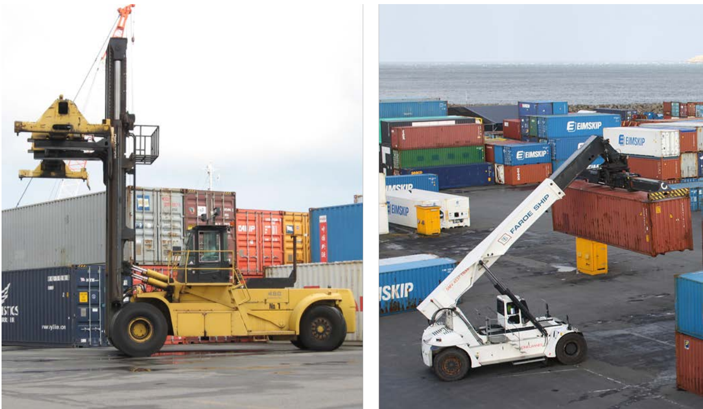
Figure 4.18: Container handling equipment; left: toploader (by Gazouya-japan is licenced under CC BY-SA 4.0); right: reach stacker (by NAC is licenced under CC BY-SA 4.0).
