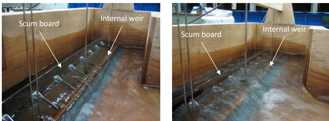
Figure 3.32 Example of a combined sewer overflow (CSO) laboratory physical scale model. Source: van Daal-Rombouts (2017).
